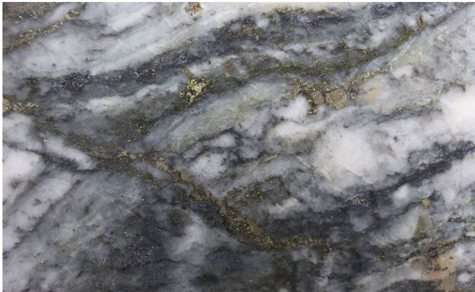
Figure 4.2 Copper mineralisation in drill core, Avoca, Co. Wicklow
