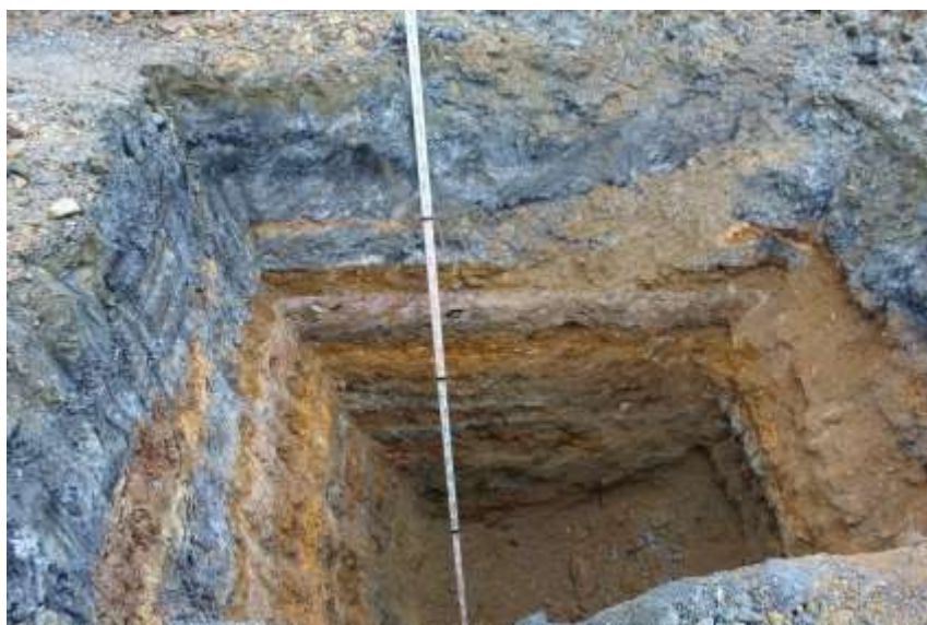
Pit sampling of the East Avoca spoil materials, undertaken in 2019 by IMC (Scale shows 4m depth of sampling)
